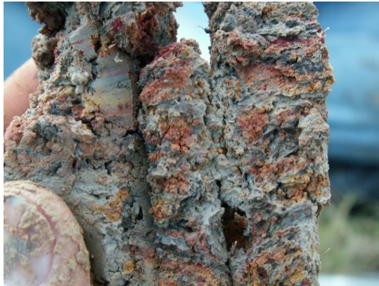
Figure 2: Example of soil showing the combination of soil matrix and mottle colours that are indicative of poor drainage
